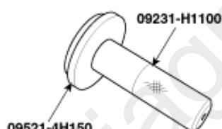
Used for installing drive pinion outer bearing
