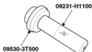
Installation of the differential side oil seal.
