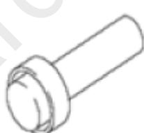
Installation of differential carrier cover oil seal.
